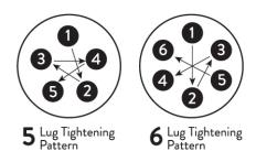
The table below outlines the torque settings for each of the braking systems/stud patterns used by AOR. Based on the recommendations presented by the various manufacturers, AOR suggests that our customers tension their wheel nuts somewhere between the wheel manufacturers guide and the hub manufacturers torque setting @ 80% of max.
