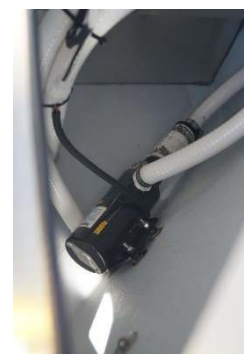
The Waste Pump installed inside the front Boot
