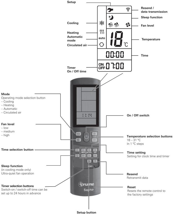
**Setup button** Tuning the remote control and the IR receiver
