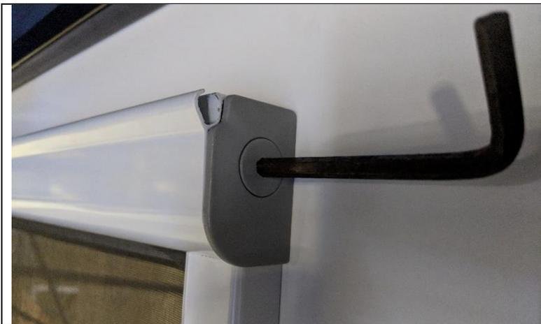
Rotate 6mm Allen key anti clockwise, taking care to keep pressure against the plug so as not to pull the spring out of container.
