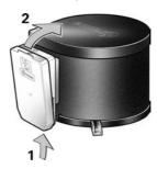
If the water heater is not to be used for a longer period, mount cowl cover (non-observance of this point can lead to the function of the appliance being impaired through water, dirt or insects), close stop cock valve in the gas supply line and close the gas cylinder.
