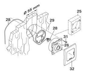
Drill a hole with diameter 55 mm.
