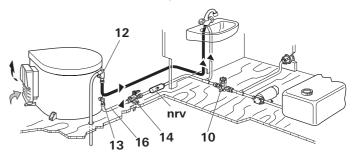
The supplied water connectors (12 + 13) and safety/drain valve (14) have a 12 mm rigid piping connection (e. g. John Guest System). For connecting to rigid pipes with other diameters appropiate adapters (not included in scope of delivery) must be used.
