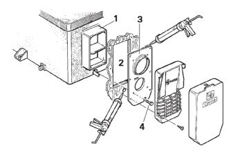
4. Remove sealing frame (3) and coat with non hardening mastic on the side facing the vehicle – do not use silicone!
