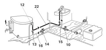
Produce connection (16) for cold water supply between safety/drain valve (14) and elbow (13 – lower pipe) on water heater.
