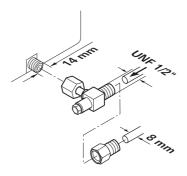
For connection to 8 mm steel piping Truma povides an adapter UNF 1/2" x RVS 8, part no. 70020-02700.
